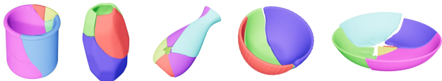
Figure 6. Qualitative results of CRAG on FRACTURA (Li et al., 2025a), demonstrating robustness on real-world fractures. All parts are real scanned fragments; colors are rendered for visualization.
