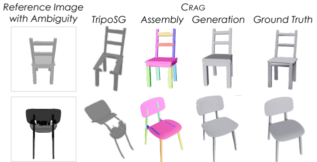
Figure 5. Qualitative results under ambiguous reference images on PartNeXt (Wang et al., 2025a). We compare image-only generation with TripoSG (Li et al., 2025b) against CRAG by visualizing CRAG’s assembled parts and generated shapes alongside the ground truth. When the reference view is incomplete and does not reveal the full object, part-level evidence helps, to some extent, resolve ambiguity and yields a better shape.
